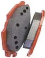
Brake linings/pad wear out due to friction, therefore regular check for cracking, glazing, contamination and wear must be conducted to ensure your safety on the road.
